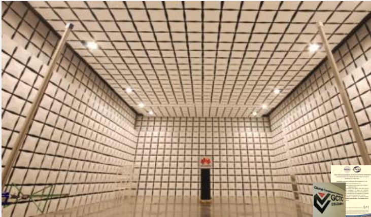
10m Radiated Emissions Test Center
