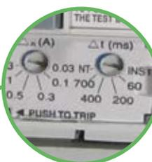
Adjustable residual current tripping thresholds between 30mA and 3A. Adjustable time delay for residual current protection between 60ms and 700ms including INST (instantaneous) and NT (No Trip).
