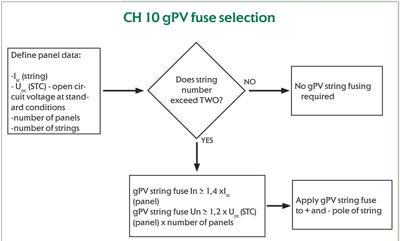
Derating factor 1,4 is defined for ambient temperature max. 45 °C .
