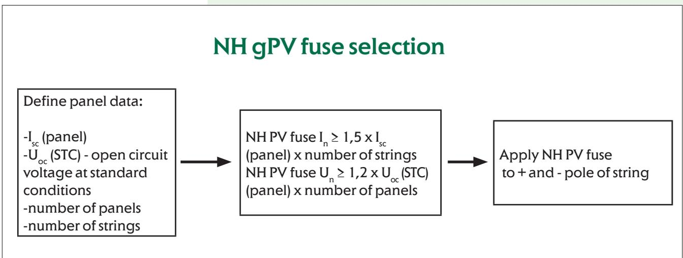
Derating factor 1,5 is defined for ambient temperature max. 45 °C
