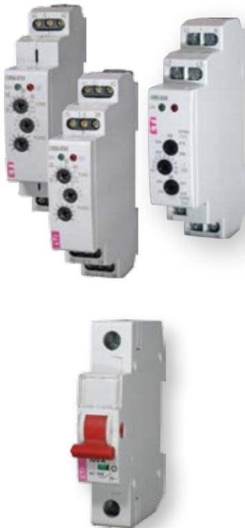
Utility grid monitoring relays HRN-54 and HRN-54N serves to monitor voltage, phase failure and phase sequence and perform anti-islanding protection together with ETI multifunction time relays CRM-91H and CRM-93H.
