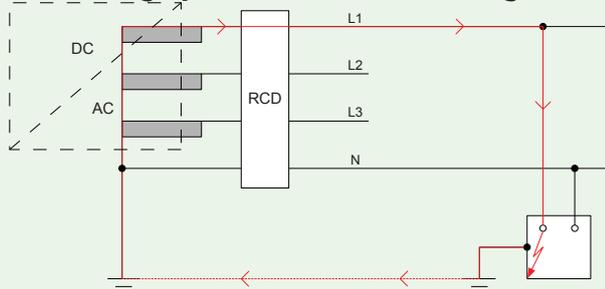
EFI type A can be used in DC/AC inverters with transformers or in DC/AC inverters for which the producer excludes the possibility of DC leakage currents on AC side.
