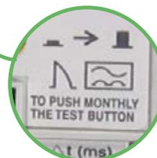
Type A: Tripping is ensured for residual sinusoidal AC in the presence of residual pulsating DC.
