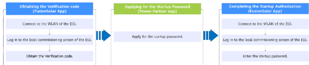
Figure 9-2 ESS startup authorization procedure
